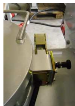
Safety switch of the sieve
