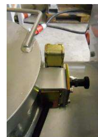
Safety switch of the sieve
