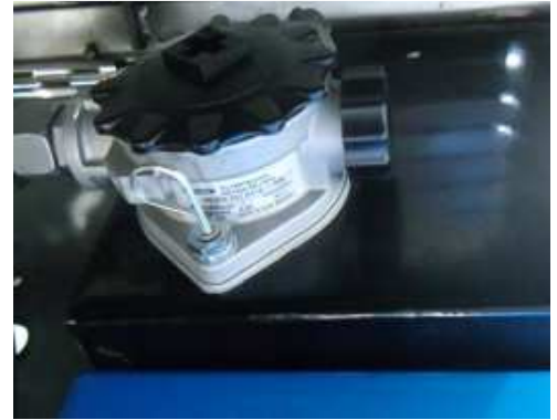
Hydraulic unit with oil dipstick and oil filler neck (black cap)
