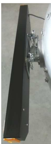
Safety pins of the rear light unit at the vessel.
