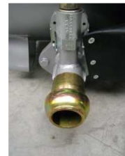
Connection for the conveyor hose at the mixing and conveyor vessel
